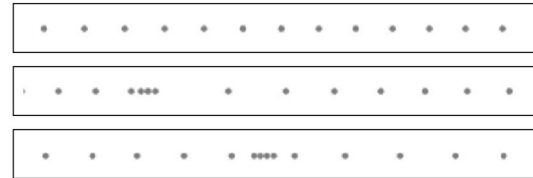
Fig. 2. Instantaneous drop positions for increasing times (top to bottom) of a system with combined symmetric and antisymmetric interactions. As shown, an initial equispaced and unstable drop array can develop a solitary propagation wave (soliton).
